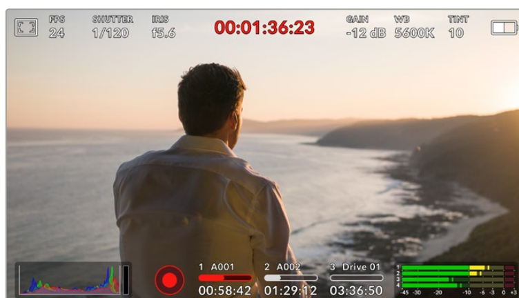
Your URSA Broadcast G2's LCD touchscreen has a comprehensive head up display and gives you easy access to your camera's most used settings
