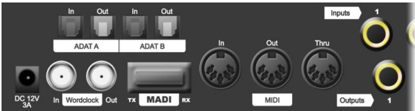
Furthermore, when using more than one A16 MK-II, it is also possible to *daisy chain* the MADI cable. In this case the device's output will be connected to the next device's input. Hence you can connect, for example, four A16 MK-II in a row in order to use the maximum number of 64 MADI channels.
