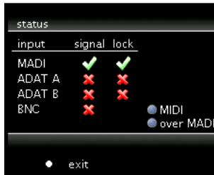
The *status screen* is a useful help when configuring the A16 MK-II, giving an overview of the digital inputs. To activate it, press **MENU** and then select *status*. The screen shows for every digital input, whether it receives a valid signal (*signal*) and whether this signal's sampling rate is correct (*lock*). Only if both conditions are met, the A16 MK-II will use the signal.
