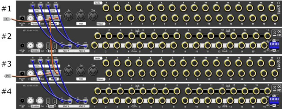
If you own two ADAT converters (in this example the A16 ultra by Sonic Core), you can incorporate them as shown. In doing so, set the routing for the two A16 MK-II as follows:
