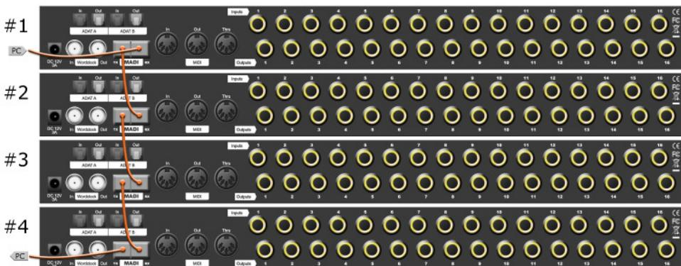
In this example four A16 MK-II are simply chained in row in order to have 2 x 64 channels. For this purpose, set the four A16 MK-II from MADI 1 to MADI 4 in the *routing preset*.
