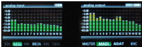
The TFT main screen shows all 32 channels of the A16 MK-II as well as the basic settings of *sample rate* and the input signal from which the A16 MK-II takes its timing. Additionally, it displays the interfaces to which the analog inputs/outputs are routed in the top right corner.
